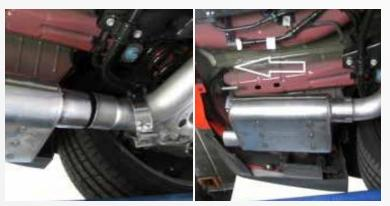
Slide the 3" band clamp and the BBK Vari-Tune Muffler onto the axle back tube. Lift upward on the muffler and hook the exhaust hanger to the chassis, reinstall the exhaust mount bolts and tighten them down.
