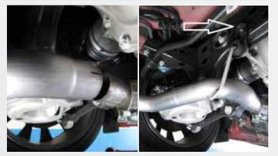
Slide the 2 <sup>1</sup>/<sub>2</sub>" band clamp and the BBK Axle Back tube over the stock exhaust pipe. Lift upward on the axle back tube and hook the exhaust hanger to the chassis.
