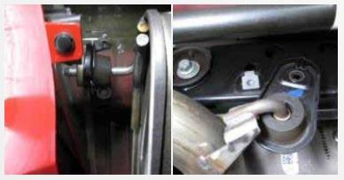
Remove the 2 bolts that secure the exhaust mount to the chassis located by the muffler tip. Next remove the bolt on the exhaust hanger that is located by the rear differential cross member. Once all 3 bolts are removed lift up on the exhaust and unhook the mounts from the chassis and remove the stock axle back from the vehicle.
