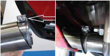
Slide the 3" band clamp onto the Vari-Tune exhaust tip with the bolt and nut facing towards the center of the vehicle and slide the Vari-Tune exhaust tip onto the outlet pipe of the BBK Vari-Tune muffler.
