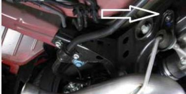
Level out the muffler and adjust the exhaust tip to your liking. Reinstall the exhaust mount bolt for the axle back tube and tighten it down. With everything in place and adjusted tighten down all exhaust clamps.
